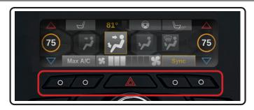
If popups are turned on in the menu: The proximity sensor, within the dash bezel, will display the descriptive tabs when your hand is near the buttons. When your hand is removed, the tabs will disappear.
