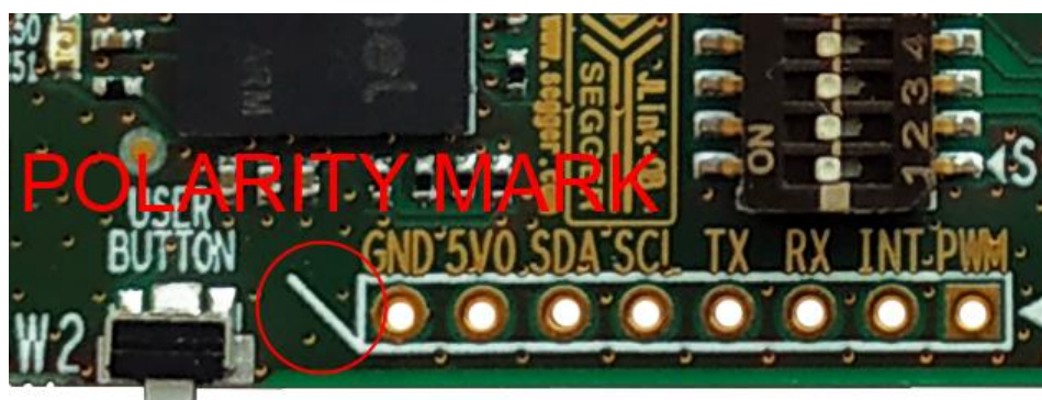
Figure 18: Guides for Proper MikroBus™ Click Board Insertion
