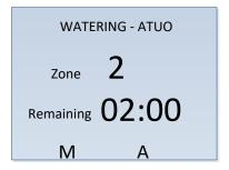
Eq.: Zone #2 is sprinkling now and the remaining sprinkling time is 2:00 min.
