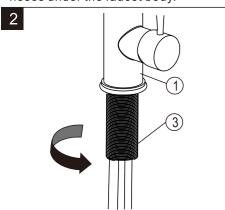
1. Make sure fasten the thread pipe(3) to the base of the faucet body clock-wise.
