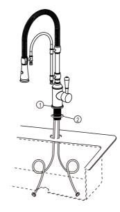
1. Make sure attach the O-ring(2) to the base.
