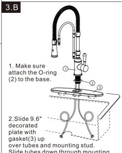
Slide tubes down through mounting hole and faucet, 9.6"decorated plate with gasket on sink.
